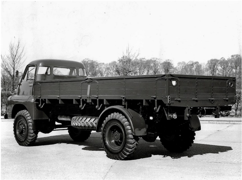
Papworth built double drop side body mounted on Bedford RLHC 3 ton 4x4 petrol engined chassis. Right hand drive, 156 inch wheelbase. Finished in deep bronze green.
