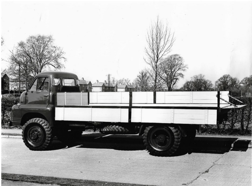
Papworth built double drop side body mounted on Bedford RLHC 3 ton 4x4 petrol engined chassis. Right hand drive, 156 inch wheelbase. Finished in deep bronze green.
